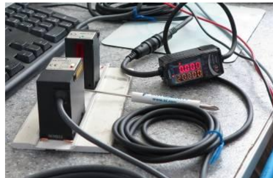
Figure 9. Testing of the ZX-GT28S4 prior to integration
