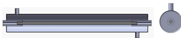
Figure 1. Cylindrical UV reactor with one centrally positioned UV lamp, for sugar syrup UV treatment, with predefined quality and concentration, low capacity
