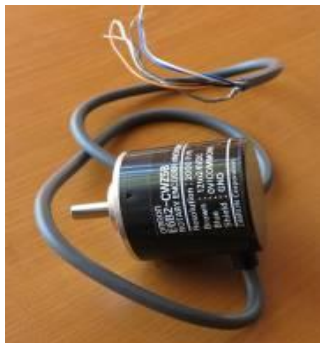
Figure 12. The E6B2 during functionality testing
