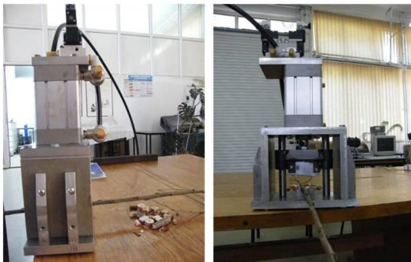
Figure 16. Testing of the cutting mechanism (side and front views)
